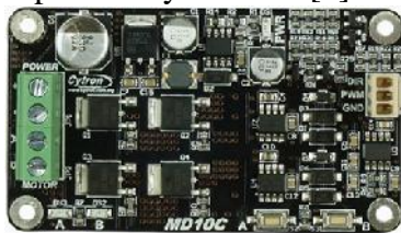
Gambar 9. MD10C dc motor driver[4].
